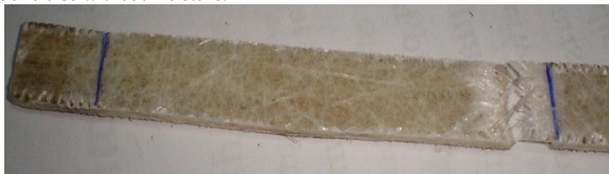
Fig. 4.1(c). Fracture due to Tensile Load
