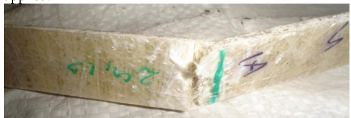
Fig. 4.7. Fracture due to Flexure Test
